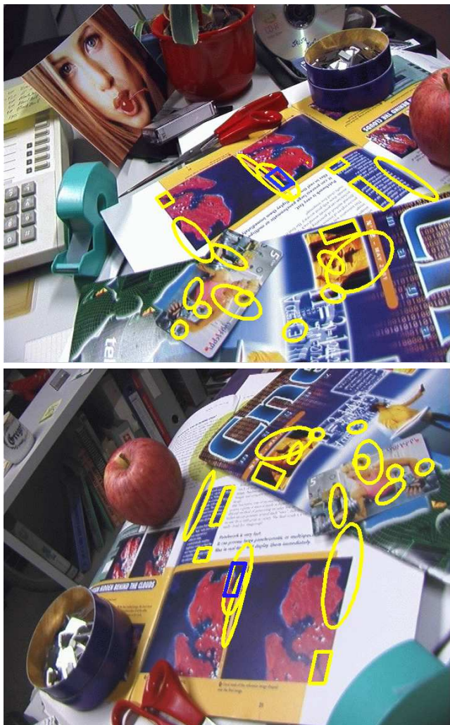
Figure 6. Invariant regions that were extracted for the images in fig. 5. Only regions are shown for which a corresponding partner in the other image has been found, but the regions in the two images have been extracted without knowledge about the other image.
